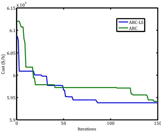
**Fig. 3.** Cost convergence for PD = 1000 MW.
